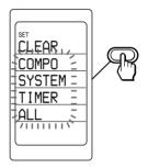
"SYSTEM" appears on the LCD display, and the system macro numbers are displayed on the labels. To change the labels (SONY OFF, SYSTEM2- 12), press the SCROLL button repeatedly. Executing a Series of Commands — System Control Functions (continued)
